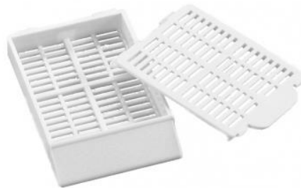
Figure 2.15. Equipment and molds used for tissue embedding. A) Leica EG1150 H Heated Paraffin Embedding Module; B) Cassettes used to hold tissues and paraffin; C) Tissue embedded paraffin blocks for sectioning.
